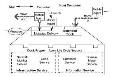
Figure 1. Mobile Agent Architecture. Mobile agents use services provided by the dock to efficiently travel through the network and, at their destination, manipulate data.
