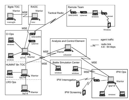
Figure 2. MI Exercise Automation Plan. Information is pushed and pulled from CI, IPW, and LRS collection teams to analysts.
