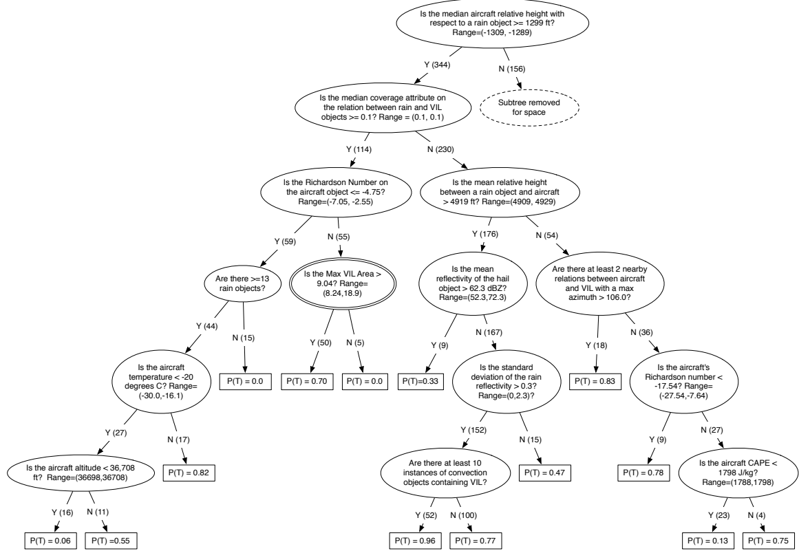
FIGURE 10. Left most subtree of the most highly ranked SRPT from the turbulence domain for 1000 samples. The tree shows the ranges on the attribute questions. Due to space limitations, we focused on the left-most subtree. The node that is double circled is discussed in the text. P(T) denotes the probability of a LMOG turbulence event.
