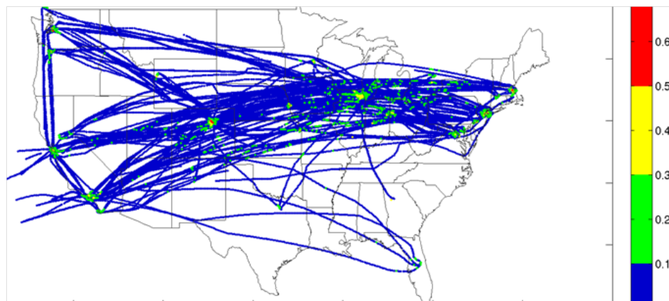
Figure 4.6: Map of eddy dissipation rate (EDR) collected by the automated turbulence reporting system on airplanes over a 24 hours period. 4
